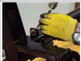
3) Unscrew the Lift Screw out of the Bronze Nut #28 in the Carrier Assembly #30, by turning the Crank Handle counter-clockwise.
